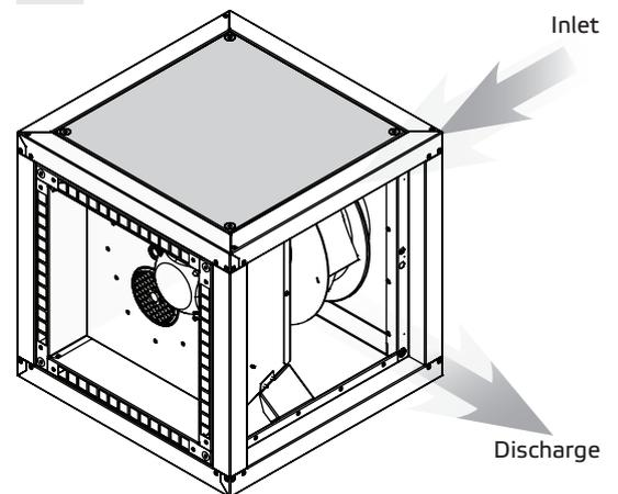
By closing an open side, the discharge side can be changed.
