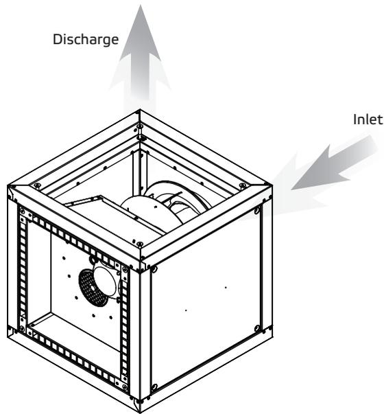
**B** In order to change the discharge side, the panels or a panel must be removed.
