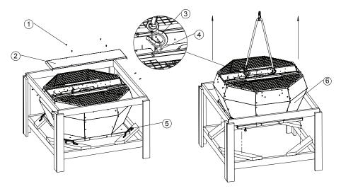
Lift the roof fan out of the packaging:
