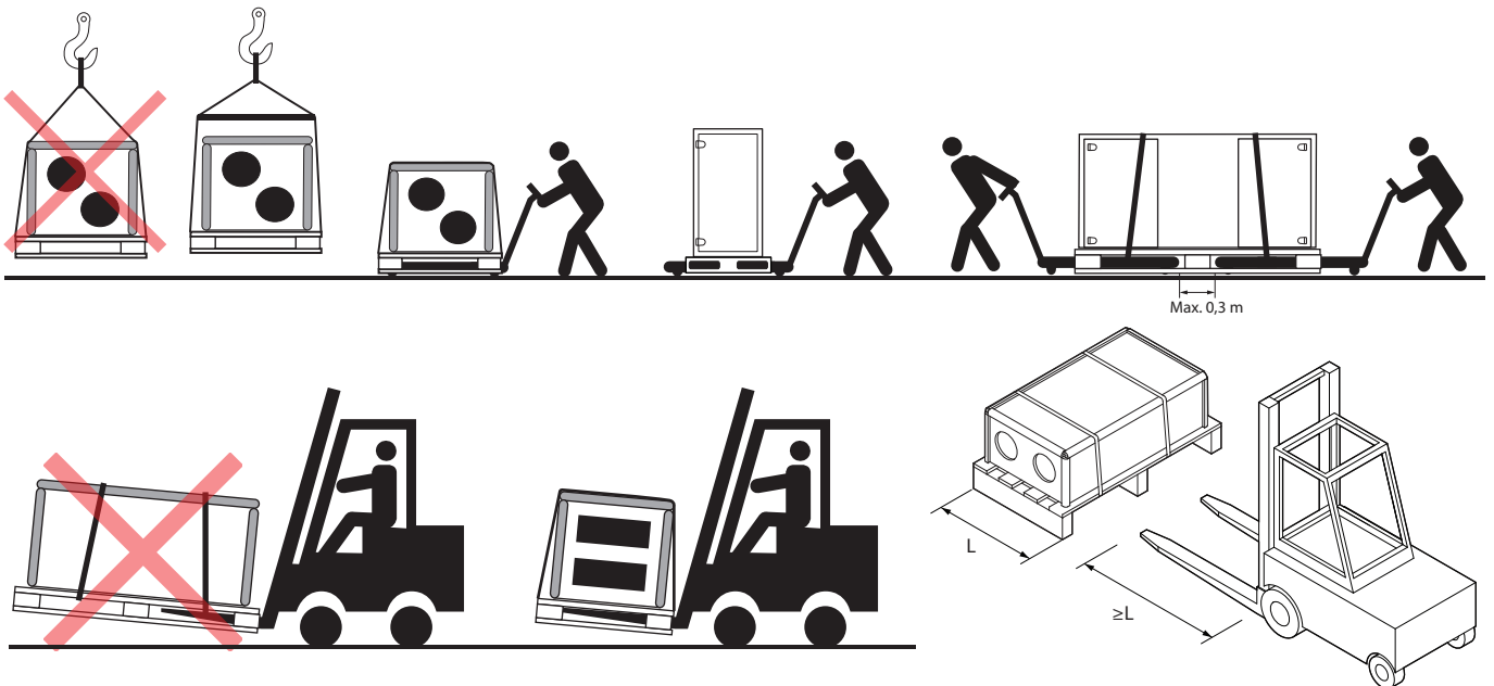
Fig. 5. Examples of transportation by crane, forklift and trolley
