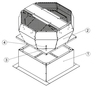
■ Fasten the roof fan (2) with screws and washers (3) and (4) on the roof socket (1)
