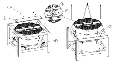
Lift the roof fan out of the packaging:
