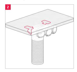
4 Fix the plenum box securely to the ceiling using the holes in the mounting wings by, for example, screws. Diameter of the wing holes is 5.3 mm.
