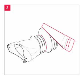
Slide the side connector on the uncovered eliptical slot. Check if the catches are properly fastened.
