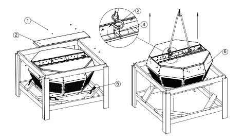
Lift the roof fan out of the packaging:
