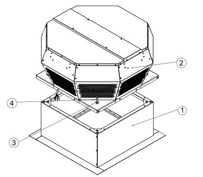
■ Fasten the roof fan (2) with screws and washers (3) and (4) on the roof socket (1)
