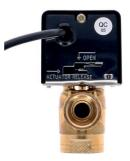
Power supply/ Frequency: 230 V AC/ 50 - 60 Hz Power consumption: 7 VA Kvs coefficient: 6.5 m³/h Operating condition of actuator: 0 - 60°C Running time (motor): 18 s Running time (return spring): 5 s Degree of protection: IP 20
