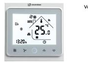
Voltage/ Frequency: 230 V AC / 50 - 60 Hz Maximum current: 5 A Operating temperature range: 0 - 45°C Regulation range: 5°C - 35°C Regulation accuracy: ± 0.5°C Communication: RS485 Dimensions: 86 × 86 × 13.3 mm 270 g Degree of protection (housing): IP 20
