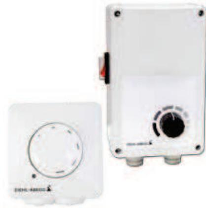
These devices for continuous speed control of one or more voltage-controlled 1~ fans have a knob installed at the front. This knob sets the desired speed. The speed controller starts with maximum output voltage for safe start-up of the fan.
